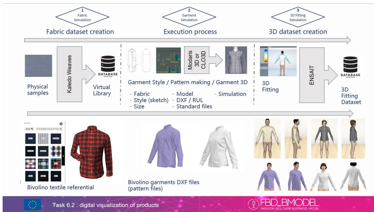
Figure 4: The complete digitalization process for textiles and garments
